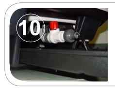
Pull the drip pan out about halfway and slowly open the discharge valve. Drain the remaining water into the drip pan and pour the water into a drain or sink. Repeat this until there is no more water draining out. Once this is done, close the discharge valve handle.
